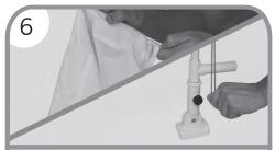
6. Slide pole sleeve of flag onto the Flexible Fiberglass Rod. Attach Bungee Cord to grommet on flag using Spring Snap and stretch bungee around thumb screw located on the Pole Holder Bracket.
