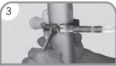
3. Attach Pole Holder Bracket to a desired pole using Stainless Steel Bands. Tighten with a 5/16" wrench or flathead screwdriver. Excess Stainless Steel Band may be removed with tin snips.
