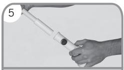
5. Insert the bottom end of the Fiberglass Pole w/Rotating T-Connector into the free Pole Holder Bracket. Hand tighten the black thumb screw to secure.
