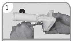
1. Locate the 2 Pole Holder Brackets and loosen the nut on each using a 1/2" wrench. Only loosen to a point where the angle of the Pole Holder Bracket can be changed freely.
