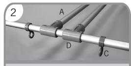
Screw the Upper Banner Arms (C) with their pre-mounted Parallel Connectors (D) onto the ends of the Distance Pieces (A).
