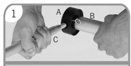
Slide pole clips onto Aluminum Pole (B). Place the Black Pole Top (A) onto the top of Aluminum Pole (B). Screw Banner Arm (C) onto Black Pole Top (A).
